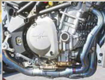
173BHP engine comes from the F4 Tamburini
