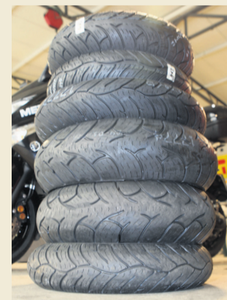
Tiny grooves in Wintecs help tyres warm up fast
