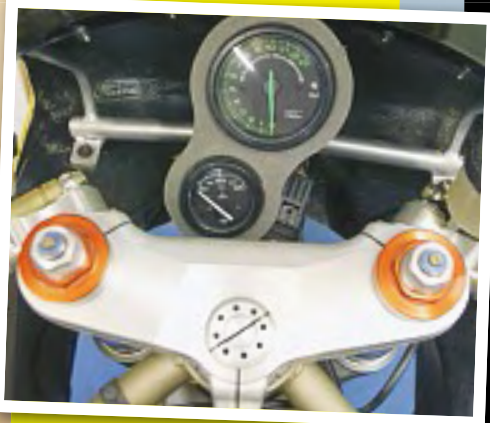
FAIRING bracket from SES (£95) fits in neatly
