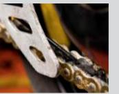
TESTER'S NOTES: The CL10 is an electronic system that reads your bike's speed and revs to work out how much oil to deliver to the chain. The dispenser uses a pressurised can of chain oil, which means you can mount the can and solenoid anywhere on the bike, but you have to use Acumen cans at £13 for three. Each can should last around 750 miles on the middle setting. The kit has two cans included.
